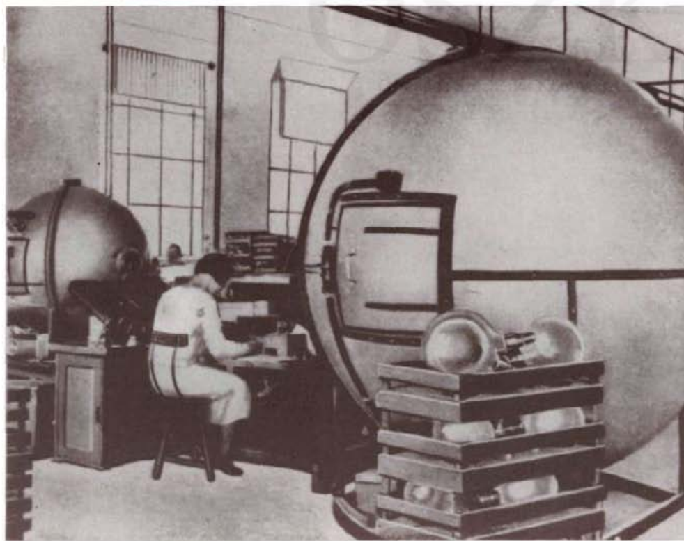
Measuring the luminosity of incandescent lamps in a photometer sphere in the 1930s.
