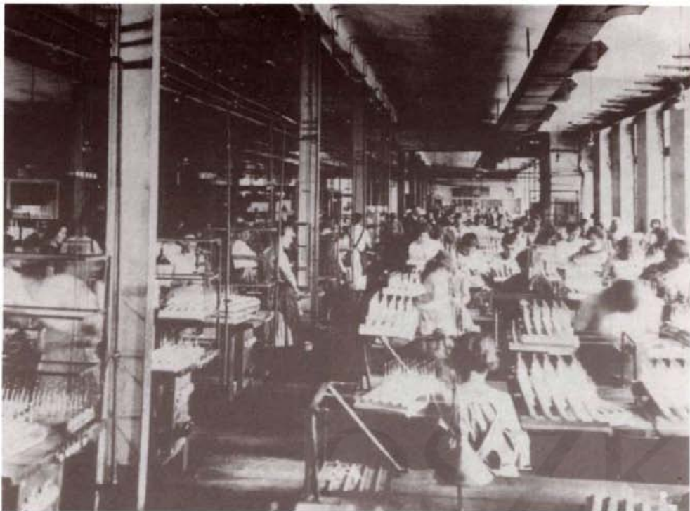
The assembling of stems with drawn tungsten filament for tungsten lamps in the beginning of the 1920s.
